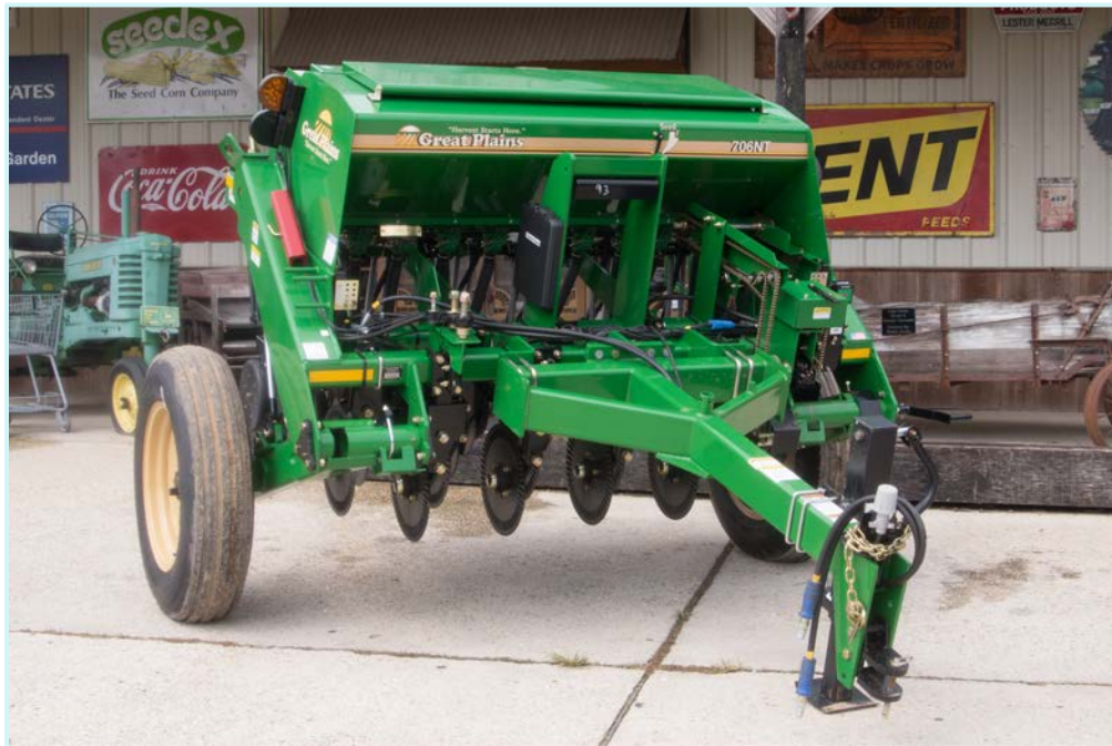
Figure 3 Seven foot no-till grain drill located at Circle T in Franklinton LA
