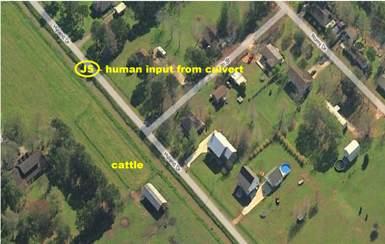
Site J5: Culvert effluent under Hyland Drive draining rear of old subdivision South of Lockport – boundary of the subdivision on south side and has pasture land in area. Large ditch drains to 40 Arpent Canal to rear.
