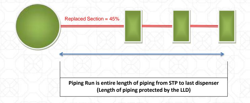
If >25% of a double-walled piping run is replaced, the entire piping run already has secondary containment so the entire run does not need replacement but interstitial monitoring is now required on the entire piping run (LAC 33:XI.507.A.7).
