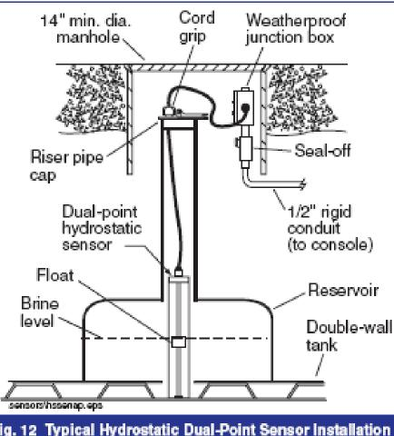
Fig. 12 Typical Hydrostatic Dual-Point Sensor Installation
