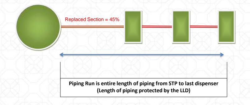
If >25% of a single-walled piping run is replaced, the entire piping run needs secondary containment and interstitial monitoring (LAC 33:XI.507.A.7).
