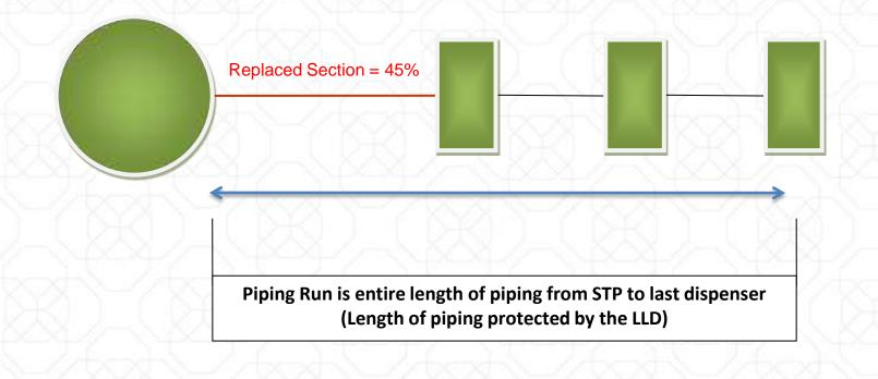
If >25% of a single-walled piping run is replaced...
