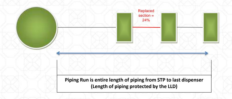
If <25% of a piping run is replaced, secondary containment and interstitial monitoring is not required.
