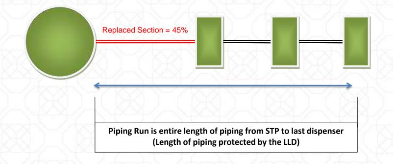
If >25% of a double-walled piping run is replaced, the entire piping run already has secondary containment...
