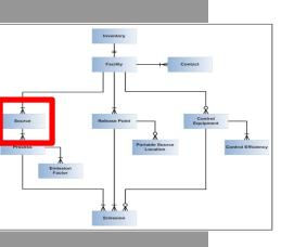
Source – Equipment or unit that generates emissions. This is the operating equipment, not the control equipment or the stack/vent
