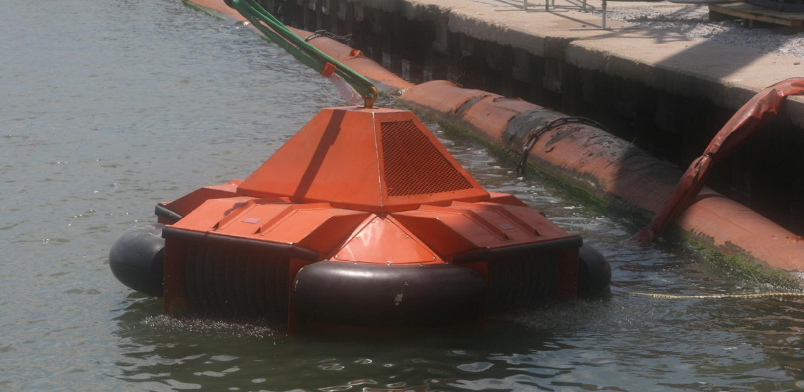
*Skimmers collect oil along the surface during a cleanup demonstration.*
