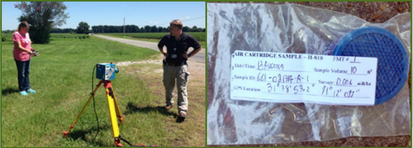
**LEFT:** DEQ Environmental Scientist Carolyn Bourn (left) takes air samples from a handheld survey meter in Tensas Parish as Environmental Scientist Michael McMahon, serving as field team controller for the drill, checks the mounted air volume totalizer. **RIGHT:** Air samples are stored in cartridges and filters which are then sealed and labeled for submission to a laboratory.
