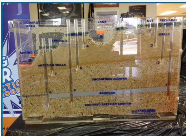
This model depicts how ground water flows and interacts with surface water, and how contaminants can migrate to water wells.
