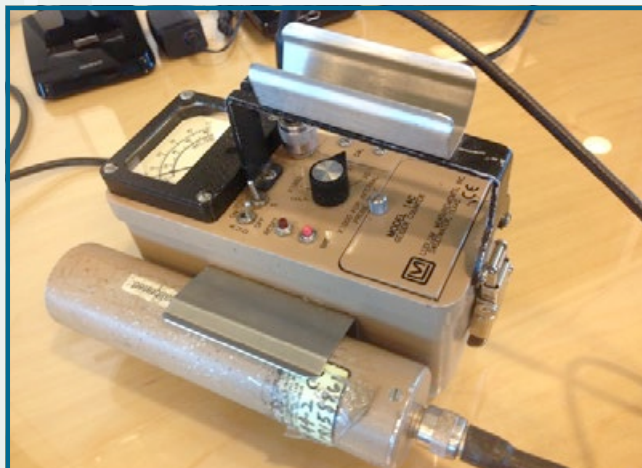
Emergency responders from LDEQ use this hand-held scintillation counter to detect the presence of radiation at a site.
