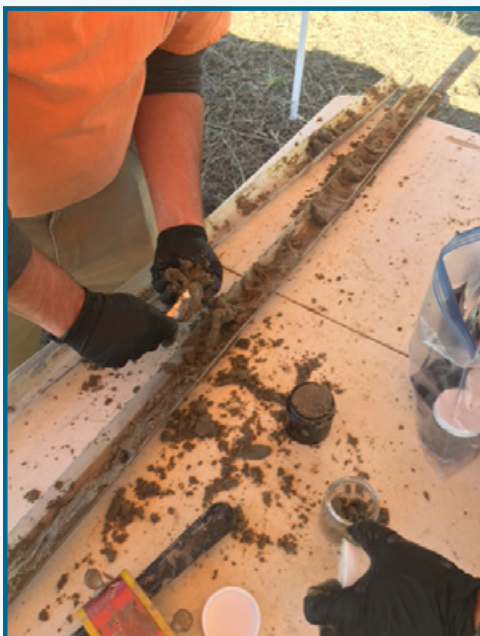
Contractors extract the soil sample from a boring device for bottling and submission to the lab.
