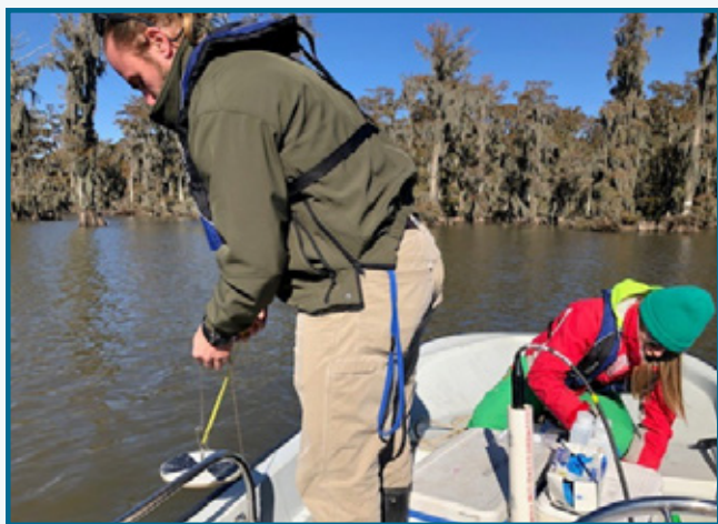
LDEQ Environmental Scientist Kyle Bird (l) deploys a Secchi disk to measure water turbidity in Lake Verret, while environmental scientist Michele Abbene collects water samples.
