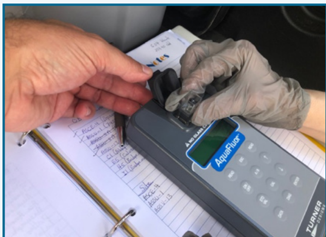
The water sample is poured into a tiny plastic vessel that is inserted into the AquaFluor meter. Optical Brightener readings are shown within seconds.
