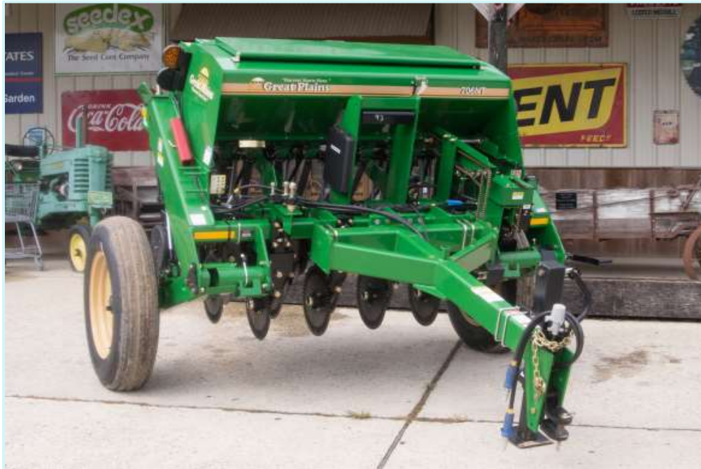
Figure 3 Seven-foot no-till grain drill located at Feed Pro in Sunset, LA
